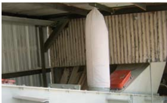
The MARTIN® Dust Bag System is available with a Standard Bag or a Static-Dissipating Bag for use in explosive environments.
