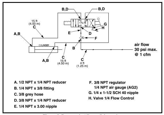
**Figure 8. Pneumatic Aligner Schematic**
