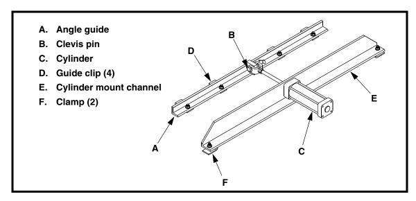
Figure 7. Installing Pneumatic Aligner
