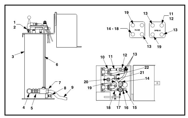
Figure 14. Boot-Lift® DBL-18 Control Console, P/N 38340X-DBL\*\*
