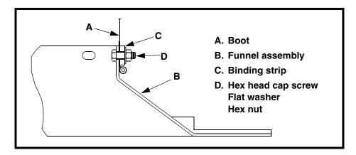
Figure 2. Attaching Boot to Funnel Assembly
