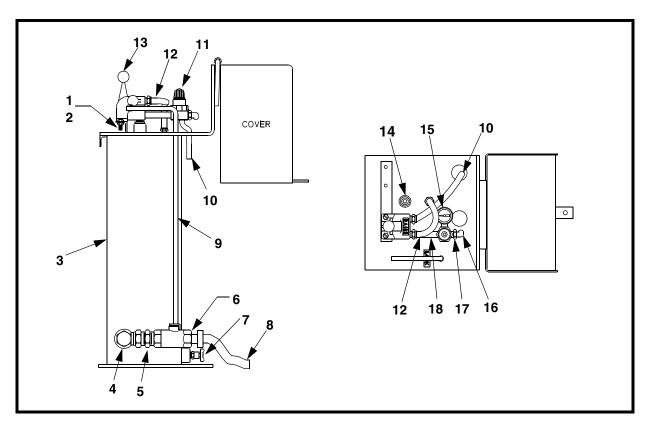
Figure 15. Boot-Lift® Control Console Assembly, P/N 38340X-SBL
