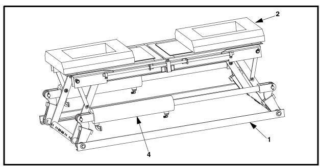
Figure 13. Boot-Lift® DBLG-18 Assembly, P/N DBLG-18XXXXX
