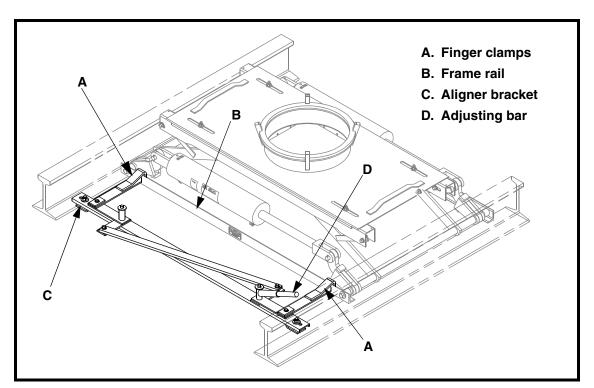
Figure 6. Installing Manual Aligner
