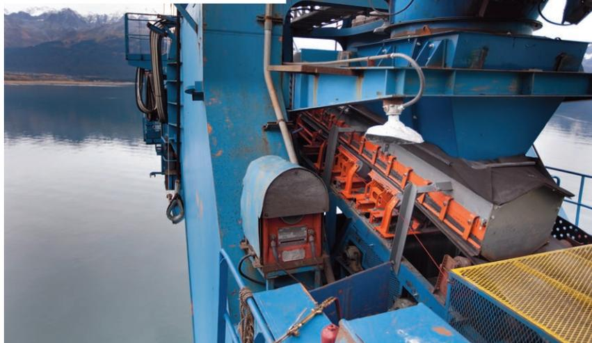
**The loading zone on the boom conveyor was recently upgraded with new components from Martin Engineering's EVO conveyor architecture, including a hood-and-spoon chute and modular belt support cradles.**
