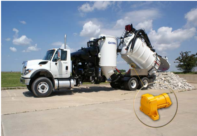
Vactor Manufacturing is employing engineered vibration to improve off-loading of industrial waste from its vacuum loaders, hydro excavators and sewer cleaners.
