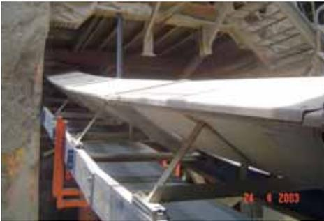
*The totally enclosed Martin® Air Supported Conveyor was retrofit onto the structure of an existing belt conveyor.*
