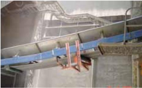
*The Martin® Air Supported Conveyor installed at Cementos Progreso was engineered with a vertical curve in the center third of the conveyor's 156-foot (47.4-m) length.*
